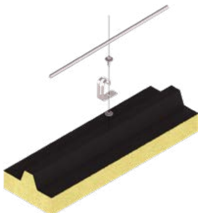
Figure 6: Installation of a suitable load-bearing element on a trapezoidal roofing.
