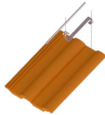
Figure 5: Installation of suitable roof load-bearing elements on concrete/brick roofing
