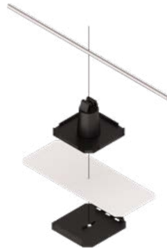
Figure 9: Installation of a SON17 A load-bearing element on PVC roofing
