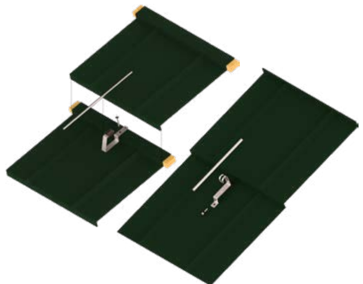
Figure 7: Installation of suitable load-bearing elements on tin sheet roofing types DECRA, GERARD, etc.
