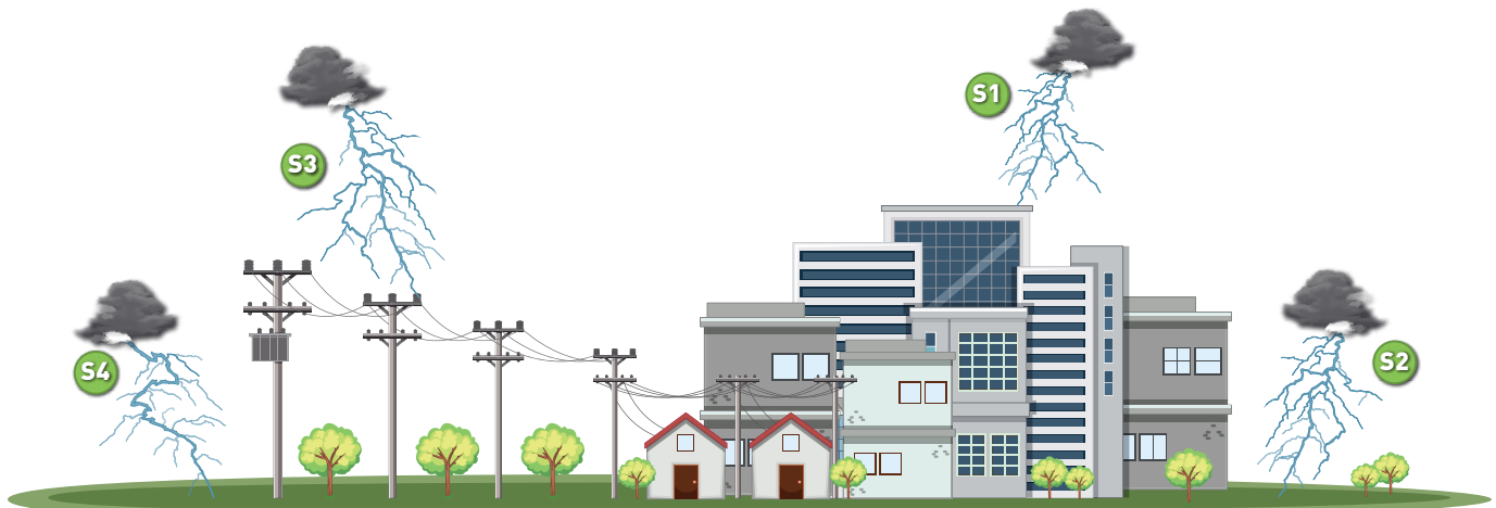
Figure 1: Source of damage according to lightning strike points
