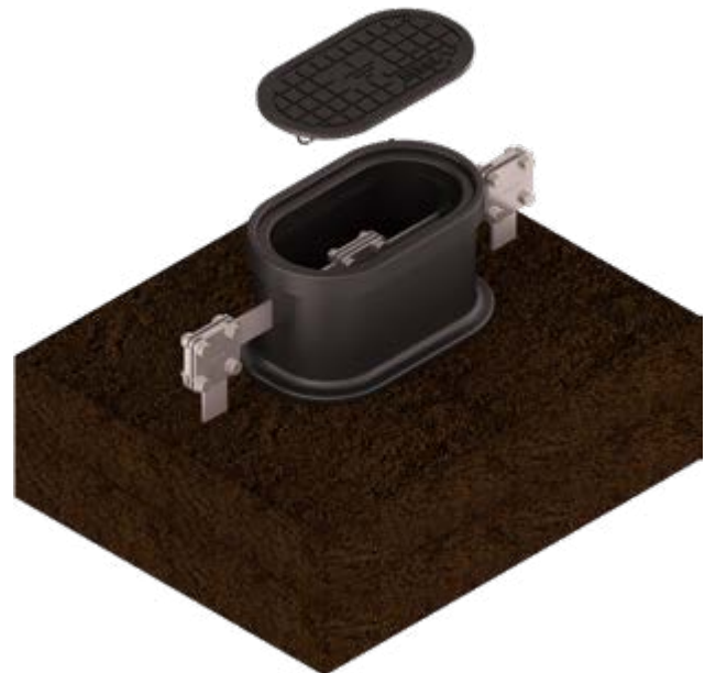
Figure 19: Installation of the measuring cabinet in the ground
