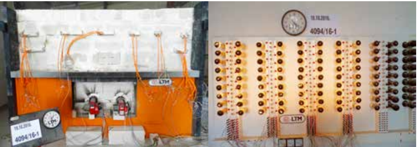
Testing of cable path system in the test chamber
