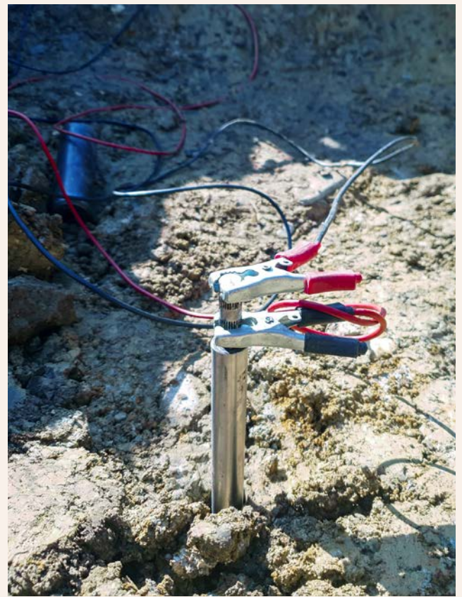
Figure 20: Example of an earthing device with a POS K Rf earth rod
