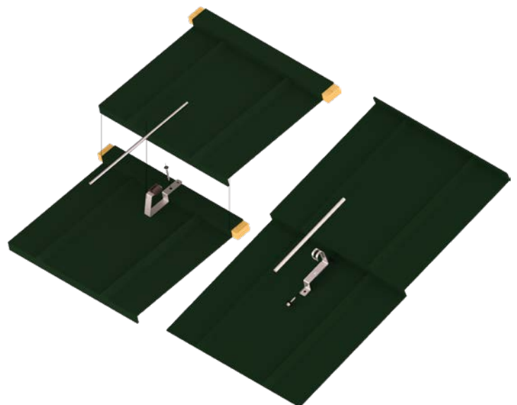
Figure 6: Installation of suitable load-bearing elements on tin sheet roofing types DECRA, GERARD, etc.
