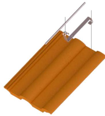
Figure 4: Installation of suitable roof load-bearing elements on concrete/brick roofing
