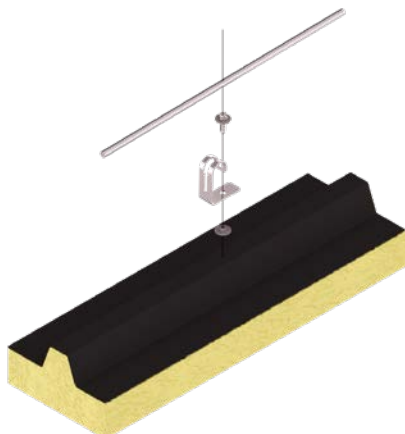
Figure 5: Installation of a suitable load-bearing element on a trapezoidal roofing.
